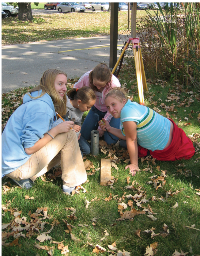
Middle school students run infiltrometer test at Edgewood College campus, Madison, WI. Photo: Cheryl Bauer-Armstrong.
