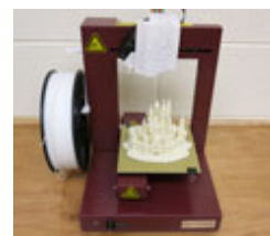
A 3-D printer and its finished product made from ABS plastic are shown. Credit and Larger Version
