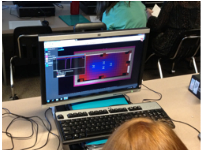
Fig. 11. This student created an interesting heater/cooler arrangement with heaters on the perimeter and coolers on the inside.
